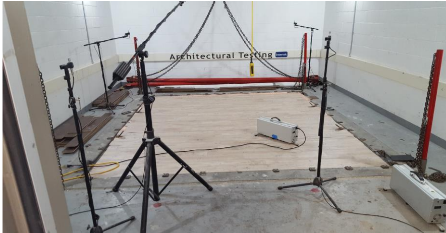
Source Room View of Test Specimen Installation
